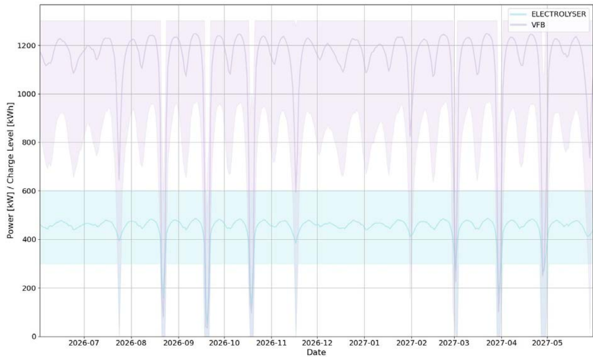
Figure 19 | HE power, VFB charge, 300 kW discharge "minimum" scheme, tidal power only.
