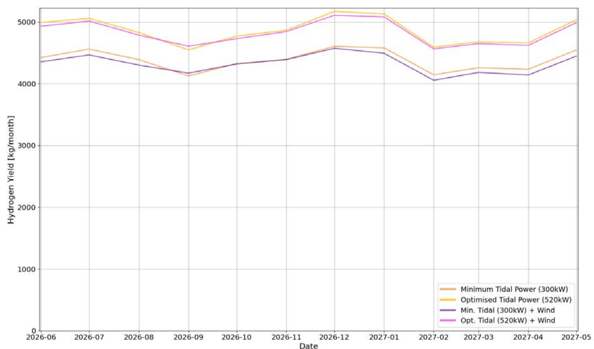
Figure 24 | Hydrogen production in kg by month “minimum” vs “optimised” schemes, tidal vs tidal + wind
